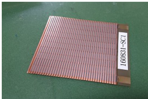
Fig. 1: Printed thermoelectric mini-generator with a mixture of Bismuth telluride and organic additives.
